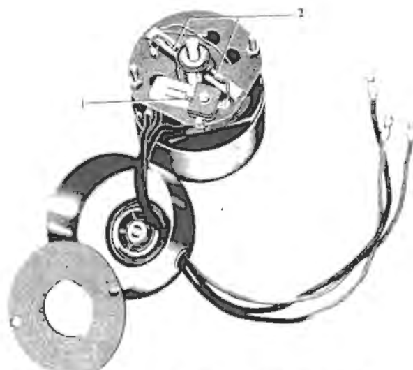
Fig. S.44.—Electric motor with cover removed.
