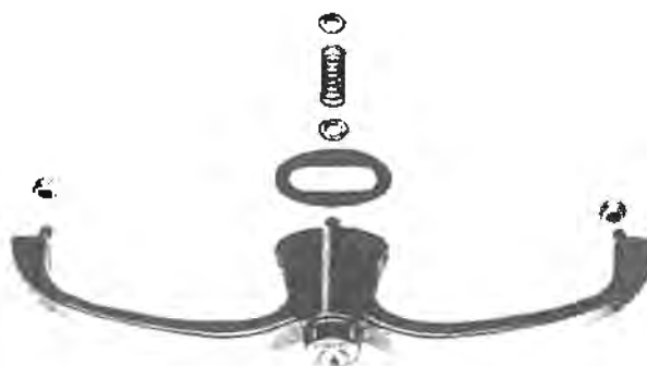
Fig. S.16.—Luggage boot lock and handle assembly.
