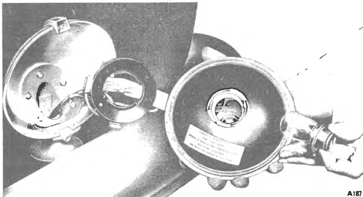
Fig. M.35.—Fog Lamp Bulb Access.
