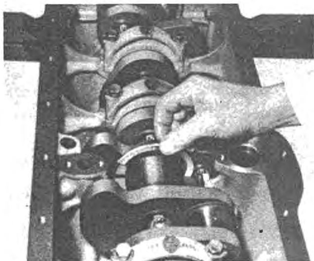
Fig. E.15.—Replacing Thrust Washers.
