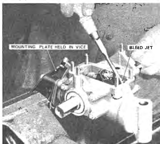
Fig. H.21.—Removing the Bleed Jets.
