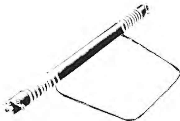
Fig. S.53.—Spring-loaded roller and nylon cord.
