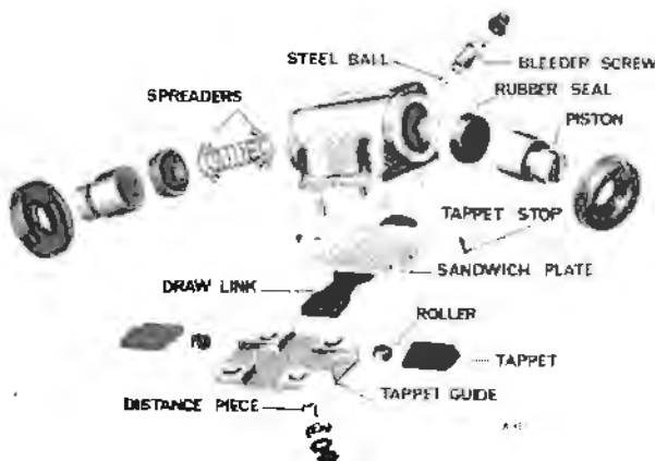
Fig. G.27.—Expander Unit—Exploded View.
