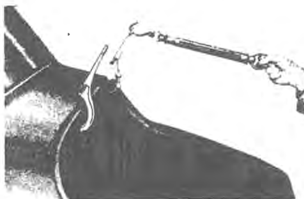
Fig. S.14.—Checking luggage boot lid assistor poundage.
