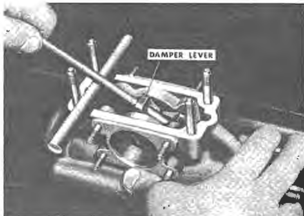
Fig. H.23.—Removing the Damper Lever.
