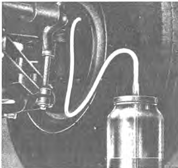
Fig. G.3—Bleeding Front Brakes.
