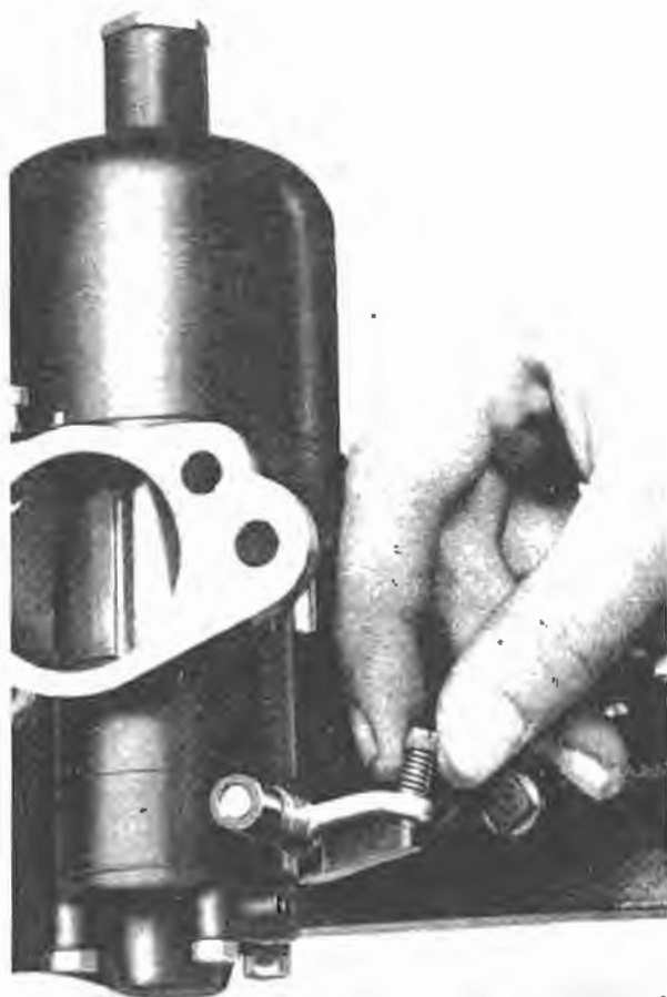
Fig. K.16.—Adjusting Mixture Control.
