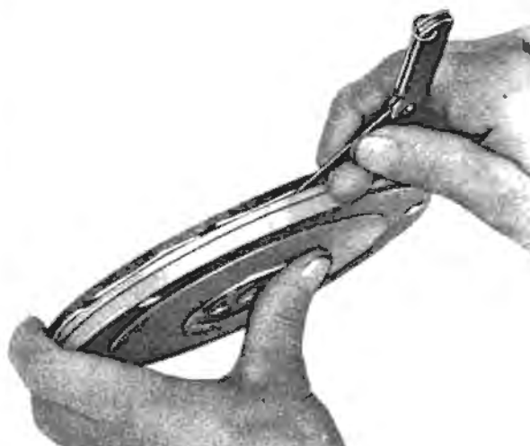
Fig. G.13.—Checking Set of the Spring Plates.
