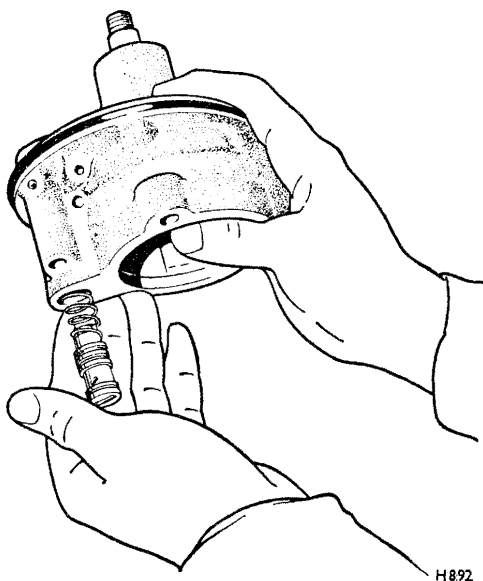
FIG. N13 REMOVING OR FITTING THE FLOW CONTROL/RELIEF VALVE
