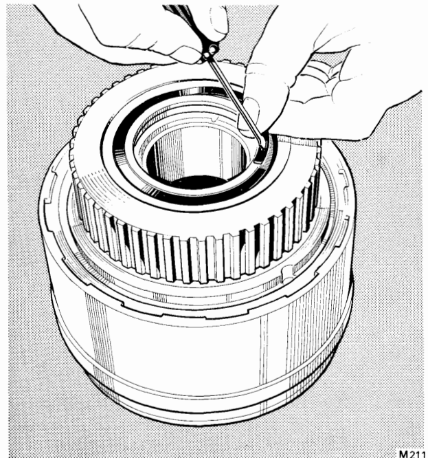
FIG. T104 REMOVING THE SPRAG RETAINING RING
