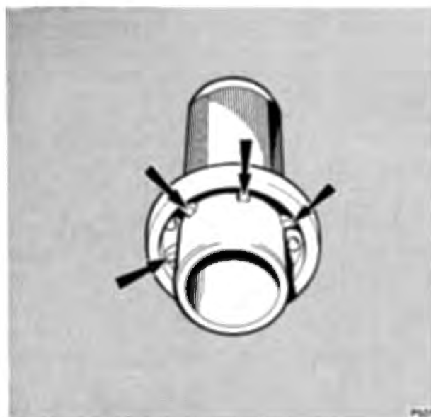
FIG. T220 UNDER CUTTING WEBBING OF SEAL INSTALLATION TOOL RH 7953 (J-21359)
