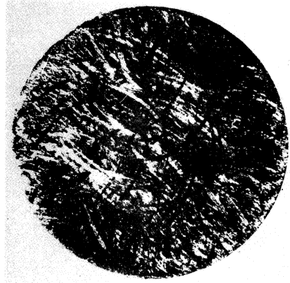
FIG. E38 SEVERELY SCUFFED TAPPET BASE
