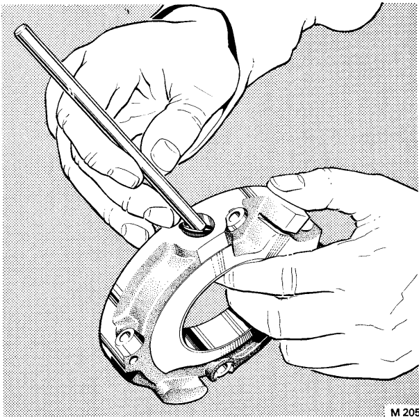
FIG. T79 FITTING THE INTAKE PIPE SEALING RING
