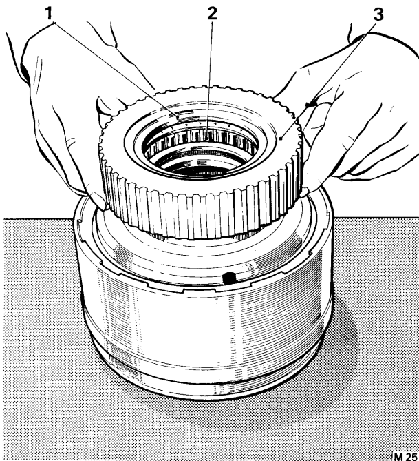
FIG. T113 FITTING THE SPRAG CLUTCH ASSEMBLY
