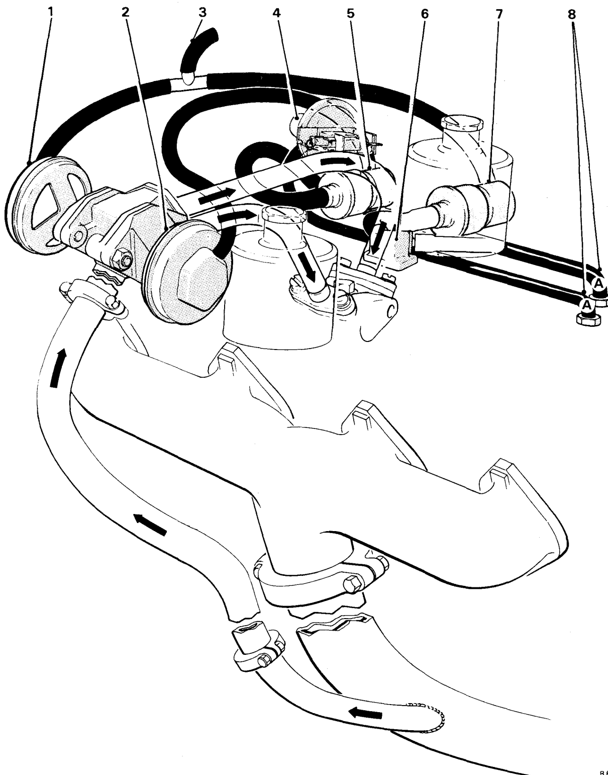
FIG. 7 EXHAUST GAS RECIRCULATION SYSTEM
