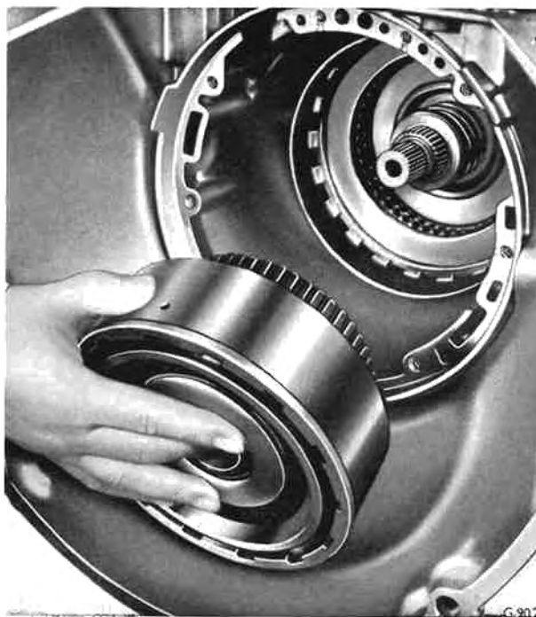
Fig. 99 Removing the direct clutch and intermediate sprag assembly
